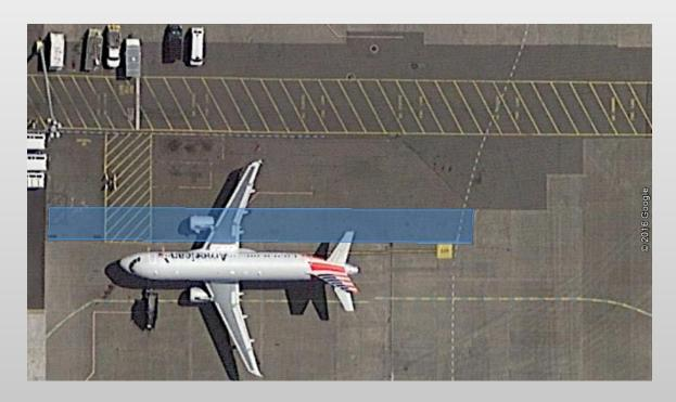
An aircraft parking at Cargo Area 2 with the right main gear on asphalt pavement not designed for such a load.
